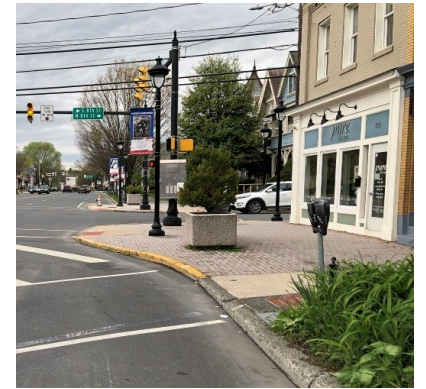
Curb Extension/Bulb- out
