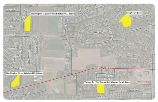
The basins will each be retrofitted to an extended dry detention basin and will enhance water quality while providing additional rainwater storage capacity. The proposed projects will include over-excavating and placing of amended soils, removal of existing low flow channels, resetting or installing stormwater outlet protection, modification of existing stormwater outlet structures, and final stabilization.
